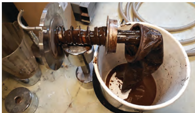
The side-stream filter's magnet and filter bag before cleaning clearly show the need for action.
